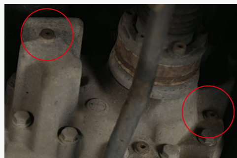
Figure 7 Note: The image above shows the oil filler/level plug locations. Haldex (left) and differential (right).
